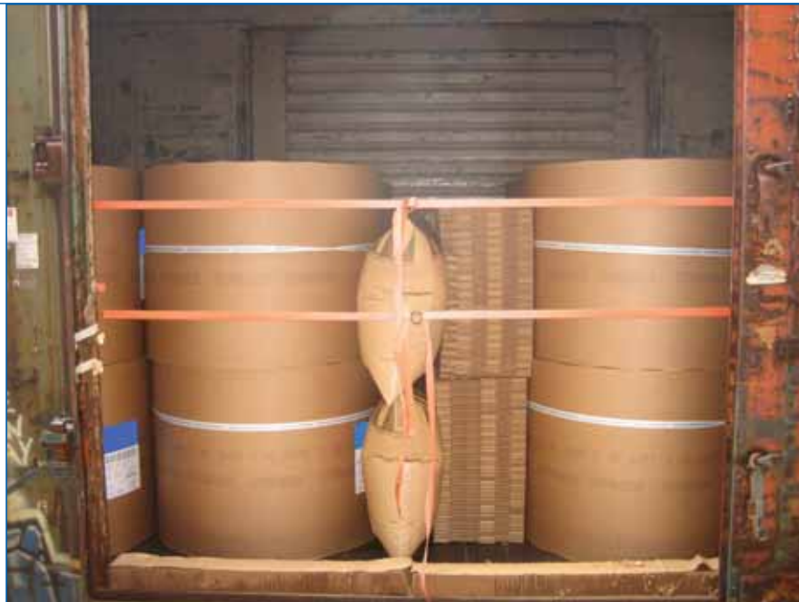
Proper Loading of 46" Rolls Photo Credit: Doug Steward
