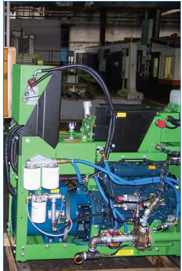
APU Awaiting Installation on Locomotive Photo by: P.M. Slaney
